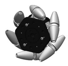
6. When building a set of 4 wheels, make sure you have 2 right handed wheels and 2 left handed. When looking at the robot from the top, the top most rollers should form an "X".
