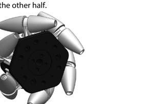
4. Secure the 2 body halves together with 3x 1.00 inch long #4-40 screws.
