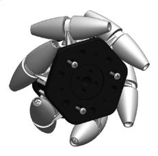
5. Flip the wheel over and add the last 3, 1.00 inch long #4-40 screws to finish the assembly.
